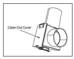
Figure 18.3 - Rear to Top Vent Adapter - 90<sup>0</sup>
